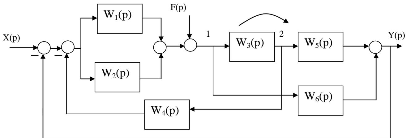
$$\text{где } W_1(p) = \frac{2}{p}; \quad W_2(p) = 1; \quad W_3(p) = 0,5; \quad W_4(p) = 2; \quad W_5(p) = \frac{1}{p}; \quad W_6(p) = \frac{2}{p}.$$
