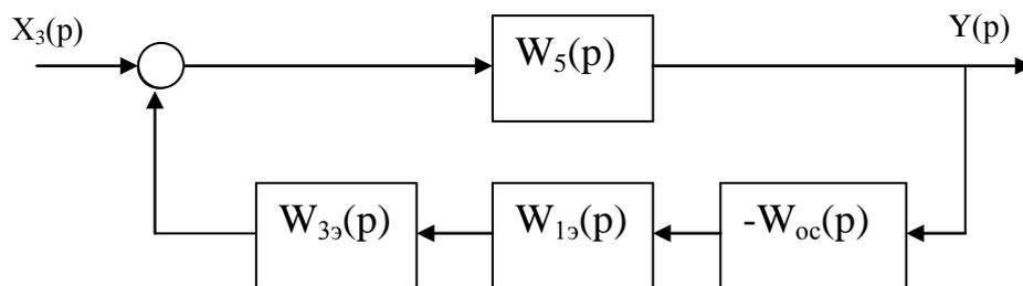
$$\begin{aligned} \Phi_{X_3Y}(p) &= \frac{W_5(p)}{1 - W_{33}(p) W_{13}(p) \cdot [-W_{oc}(p)] W_5(p)} = \frac{0,2}{1 + \frac{2(p-1)}{p} \cdot \frac{10}{p+20} \cdot 0,2} = \\ &= \frac{0,2p(p+20)}{p(p+20) + 4(p-1)} = \frac{0,2p^2 + 4}{p^2 + 24p - 4}. \end{aligned}$$
